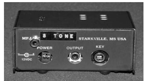
Figure 2 – Keyer Rear with Newly Installed RCA Phono Jack in Upper Left Corner
