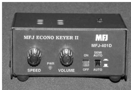
Figure #1 – Front Panel of MFJ-401D
