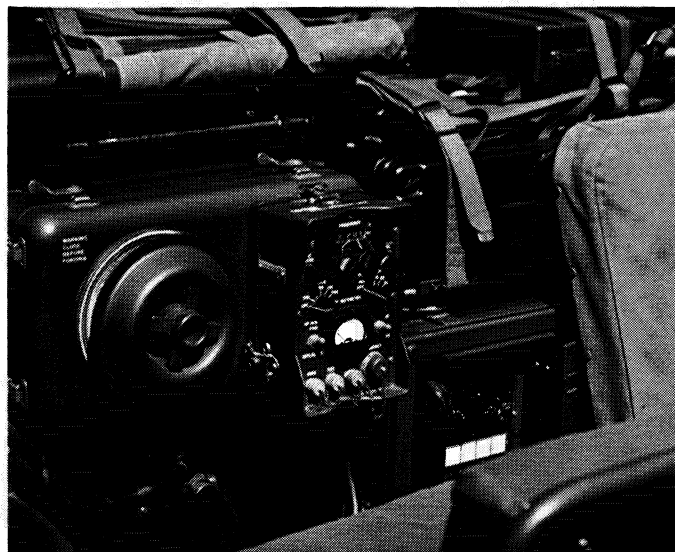
Controls are centrally located. The HF control unit may be quickly detached for semi-remote operation.
