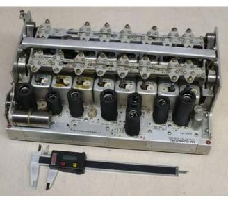
Figure 3. AM-1528A RF tuner used in the ARC-58/TRC-75. The URC-32/KWT-6 tuner is similar but manually tuned
