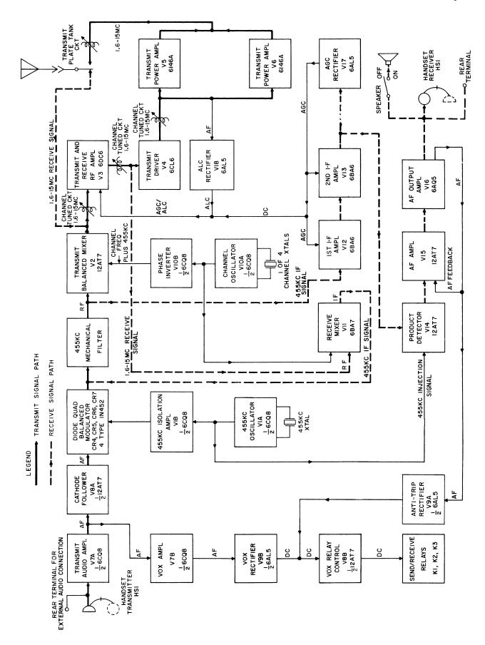
Figure 4-1. Transceiver 32RS-1, Block Diagram
