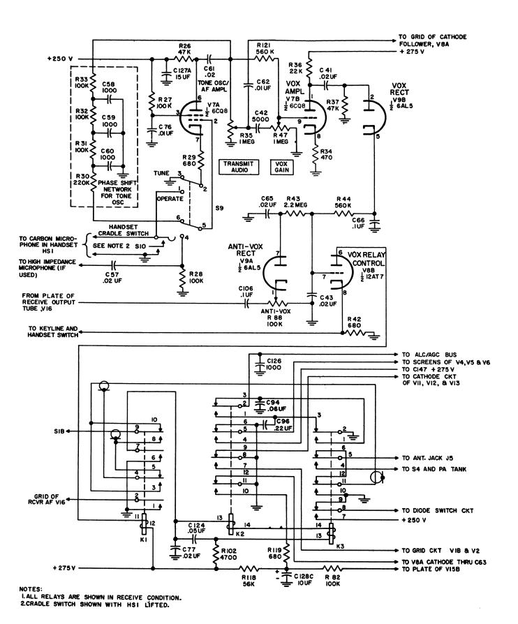
Figure 4-2. Partial Schematic, Vox Circuits
