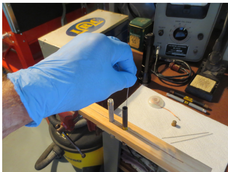
Figure 4. In the test fixture & feeding fuse wire in
