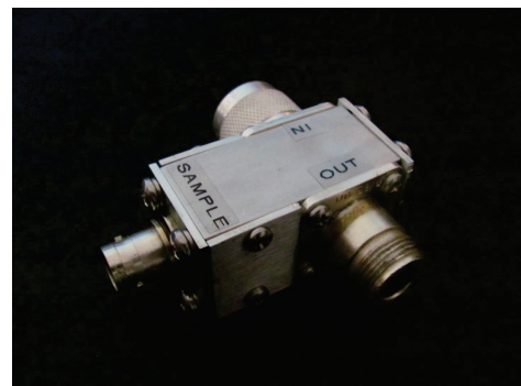
Figure 2— Don's Homebrew 50 db Sampler
