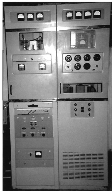
Collins T-440/FRT-24. The modulator, with dual 4-400A's can be seen through the upper left window. The RF Assembly is on the right. You can see the 4-1000A in the upper right window.
