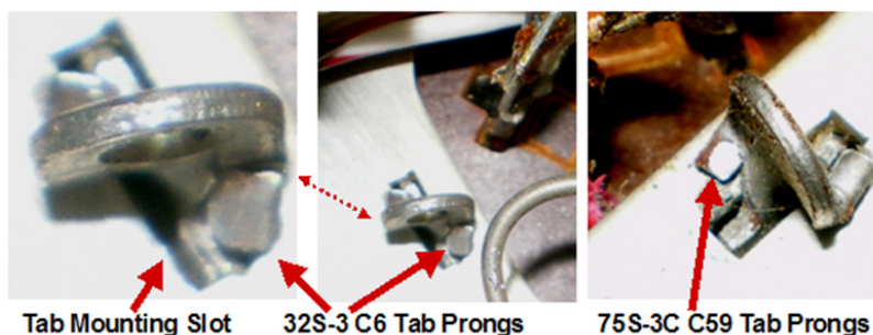
Figure 2 – 32S-3 C6 and 75S-3C C59 With Highly Deformed Prongs and Locking Tabs
