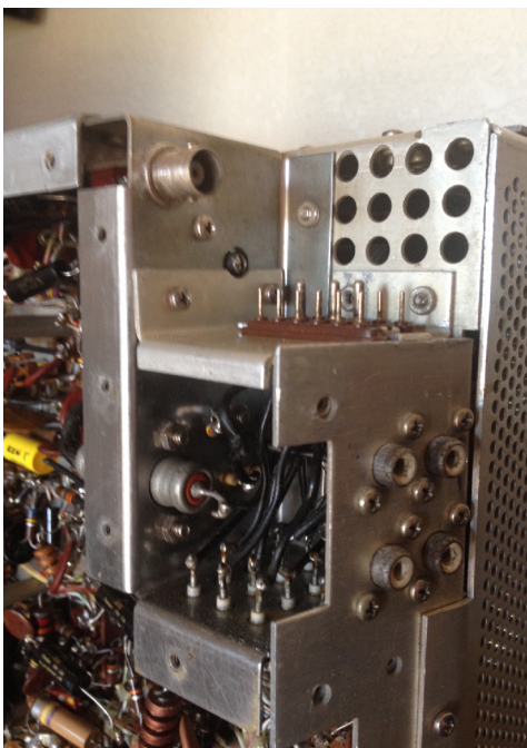
Busy Busy Busy KWM-1 Prototype Underside (Note the power plug area at the top rear left in the picture with the plug exiting to the side)
