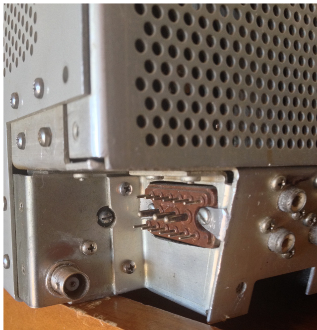
Busy Busy Busy KWM-1 Prototype Underside (Note the power plug area at the top rear left in the picture with the plug exiting to the side)
