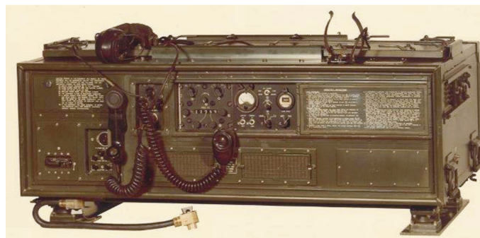
Figure 4. AN/TRC-75 HF SSB Communications System based on the ARC-58 units adapted for mobile service.
