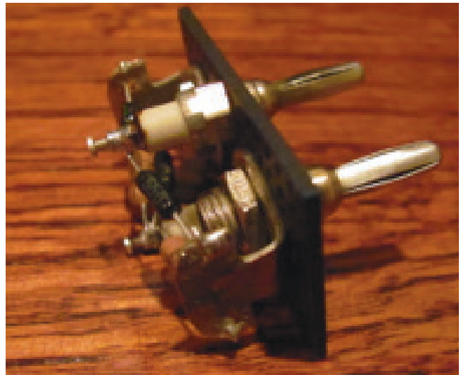
Figure 6: External 1V/3V Divider Assembly
